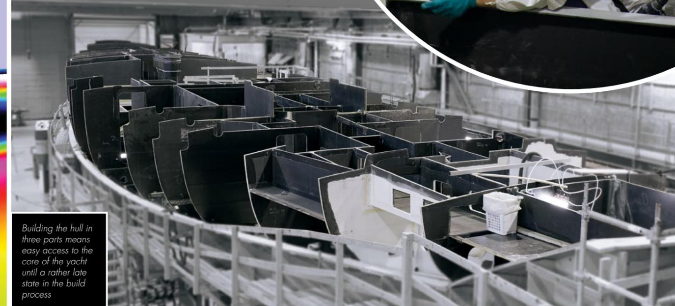
Building the hull in three parts means easy access to the core of the yacht until a rather late state in the build process
